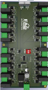
EA-DI-MCP23017-16CH I2c Address = 0x22
